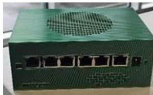
Figure 30: 5G and V2X on-board unit for the connected vehicles
