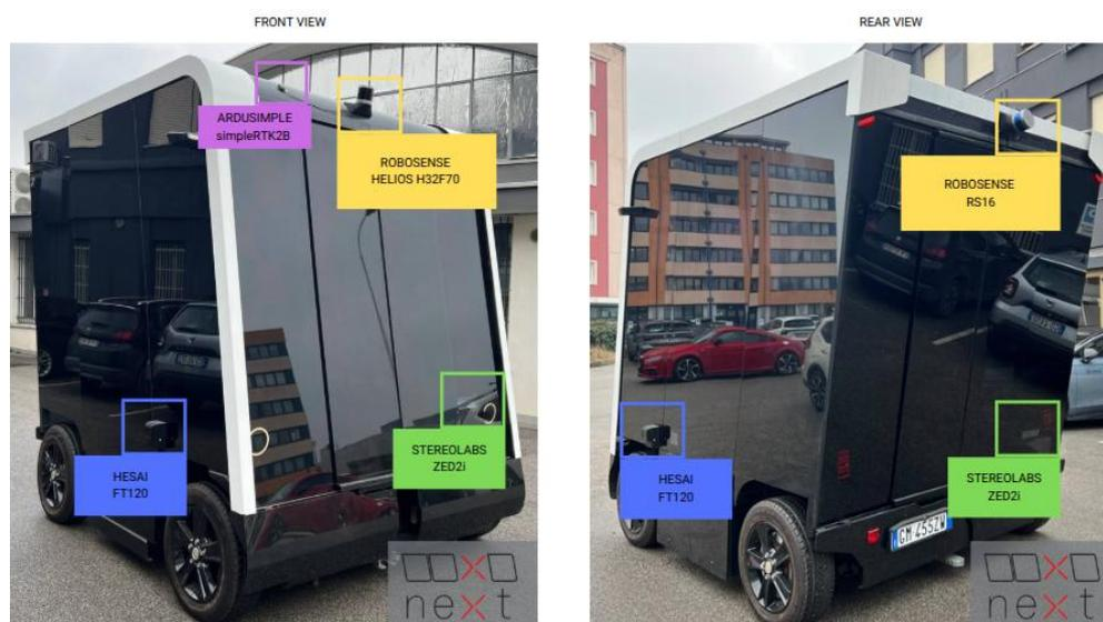
Figure 16: Sensors Placement on our prototype
