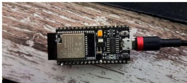
Figure 6: IoT Module using an ESP32 microprocessor
