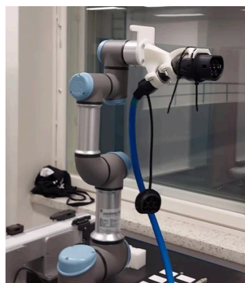
Figure 55: Phase 0 table/lab tests on-going with the University of Applied Science Lapland. This robot hand will be installed to Remoted depot in phase 1
