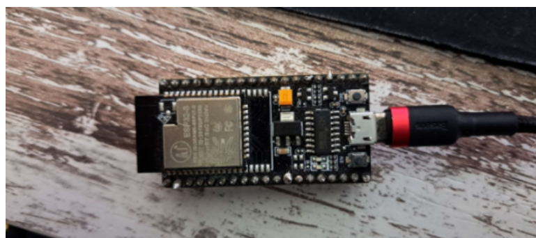
Figure 52: IoT Module using an ESP32 microprocessor
